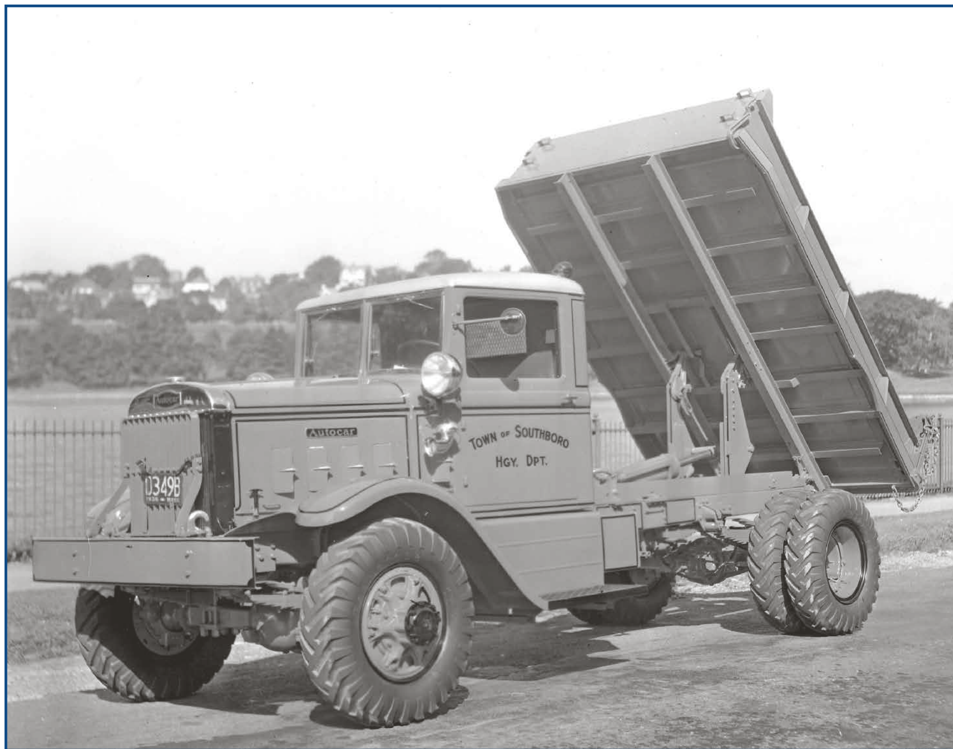
Town of Southboro, Autocar four-wheel drive dump truck, 1936
